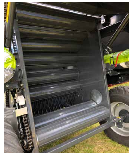
Lower main bale chamber with twin support rollers.
