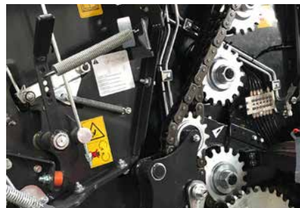
1¼" High specification 'HBC' chains are utilised on all bale chamber and rotor drives.
