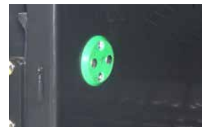
Moisture sensors located inside bale chamber.
