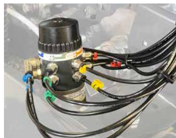
Automatic chain lubrication with individually adjustable outlets.
